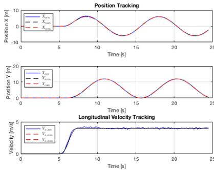
Figure 21. Circle: Position and Velocity Tracking Response
