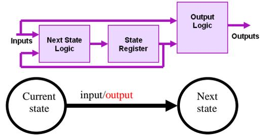
Figure 6. Principle of a Mealy machine
