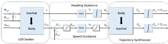
Figure 9. LOS PPG Trajectory Generation Architecture
