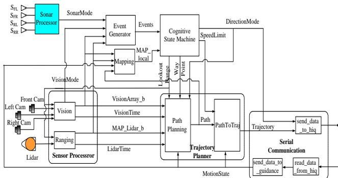
Figure 5. Cognitive Control Subsystem.
