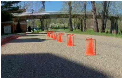
Figure 15. Vision detection (light, cone, line)
