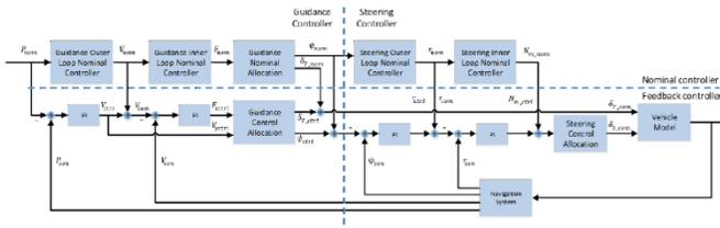
Figure 11. 3DOF Trajectory Linearization Controller Block Diagram.
