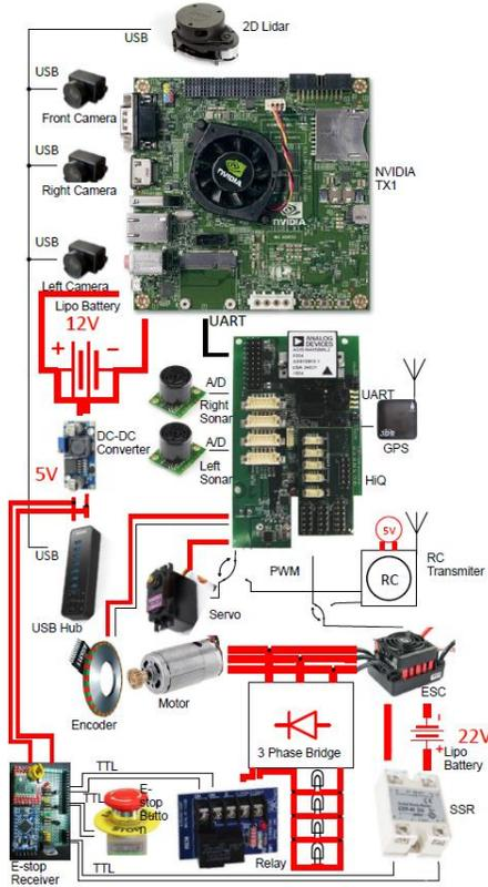
Figure 2. Electrical and Electronics Subsystem Design
