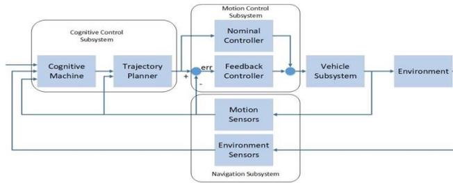
Figure 3. Autonomous Vehicle Control System Architecture
