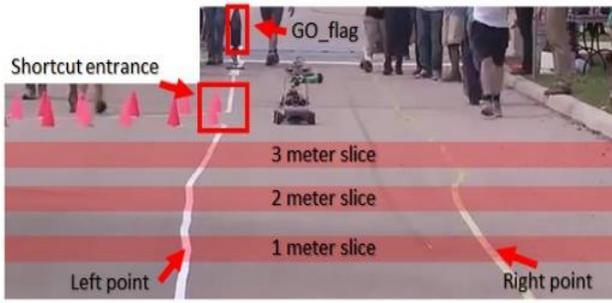
Figure 4. Example of detected lanes and objects.
