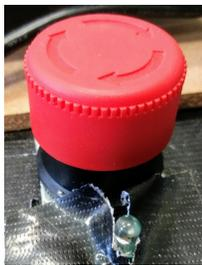
Fig. 3. Mechanical E-Stop. The motor power status is indicated by the red LED visible on the bottom of the figure.
