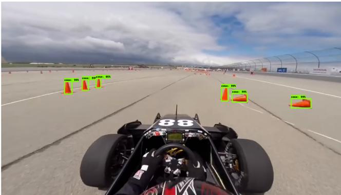
Fig. 12. Qualitative result of the cone detection network on a video.
