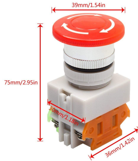
Fig 7: Emergency Stop button used for Fenrir manually activated, namely the Emergency Stops (E-stops). Physically located onboard the chassis is the E-stop tower. This metal construction sets the button at a height of around 45cm and is bright red to bring attention to itself. Upon pressing it cuts power to all components associated with the motors causing the vehicle to coast to a stop. Next is the wireless E-stop. Built off of the HC-06 Bluetooth transmitter/receiver it has an effective range of 65 ft (unobstructed view) and can be connected to a laptop or phone. When triggered it alerts the Arduino microprocessor to set the
